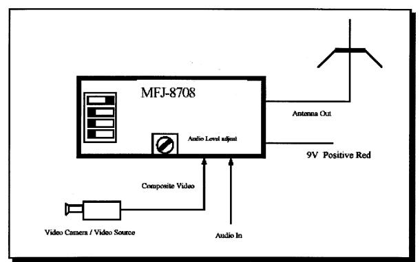
The diagram above shows the how the MFJ-8708 needs to be connected to a video and audio source. Make sure that you have SMPTE standard video at 1 V P-P. Most consumer and commercial camera's and camcorders deliver composite video, at the **''Video Out''** connector. If you are not sure if the camera is delivering SMPTE standard video, you can confirm this by looking at the video signal on a oscilloscope.
